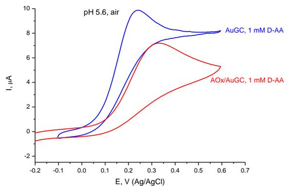
**Fig. 4.** CVs of the modified glassy carbon electrode without (blue) and with immobilized AOx (red) in 0.1 M potassium phosphate buffer pH = 5.6; in the presence of 1 mM L- ascorbic acid (on the left) and 1 mM D- isoascorbic acid (on the right);  $v = 5 \text{ mV s}^{-1}$ ; reference electrode Ag/AgCl, 3M KCl.
