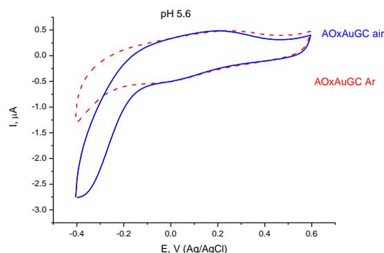
**Fig. 1.** CVs of the enzyme electrode in 0.1 M potassium phosphate buffer pH=5.6 under deoxygenated with Ar buffer (dashed line) and under aerobic conditions (solid line);  $v = 5 \text{ mV s}^{-1}$ ; reference electrode Ag/AgCl, 3M KCl.
