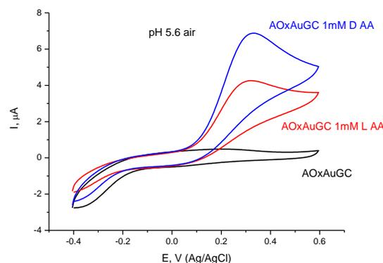
**Fig. 2.** CV of the enzyme electrode in 0.1 M potassium phosphate buffer pH 5.6 - background (black); in the presence of 1 mM D-isoascorbic acid (blue) and 1 mM L-ascorbic acid (red);  $v = 5 \text{ mV s}^{-1}$ ; reference electrode Ag/AgCl, 3M KCl.
