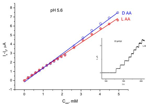
**Fig. 5.** Background-corrected steady-state response of the enzyme electrode as a function of ascorbic acid concentration at an operating potential of 200 mV (vs. Ag/AgCl, 3M KCl); stirring rate: 350 rpm; supporting electrolyte: 0.1 M potassium phosphate buffer, pH= 5.6; Inset: part of the authentic record of the current change upon addition of L-ascorbic or D- is-ascorbic acid aliquots.
