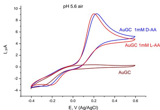
**Fig. 3.** CV of the modified glassy carbon in 0.1 M potassium phosphate buffer pH= 5.6 (black); in the presence of 1 mM D- isoascorbic acid (blue) and 1 mM L- ascorbic acid (red);  $v = 5 \text{ mV s}^{-1}$ ; reference electrode Ag/AgCl, 3M KCl.
