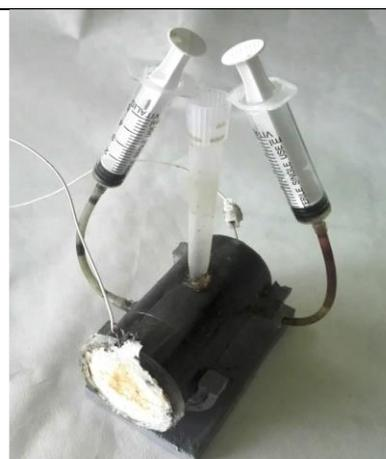
**Figure 2.** Laboratory prototype of the MFC.
