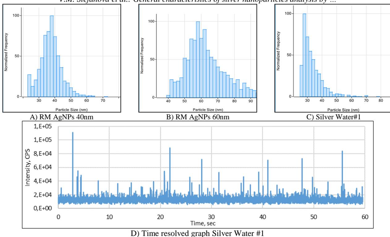
**Fig. 3.** Size distribution diagram of A) RM AgNPs 40 nm; B) RM AgNPs 60 nm; C) Silver water#1 and D) time-resolved data record for Silver water #1
