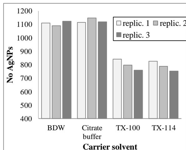
**Fig. 2.** Effect of the carrier solvent on the number of registered particles in three consecutive replicates upon introduction of RM AgNPs 60nm at a concentration of  $125 \text{ ng L}^{-1}$
