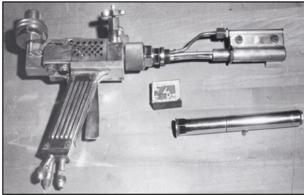
Fig.1. General view of the experimental plant in the form of a rocket flame-jet rocket burner torch
