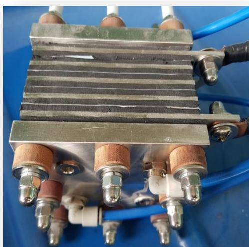
**Figure 2.** Picture of a small laboratory AEM electrolyser with 4 single cells
