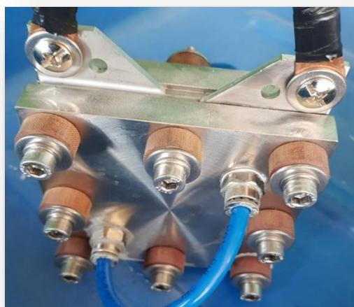
**Figure 1.** Picture of a self-designed single AEM electrolysis cell
