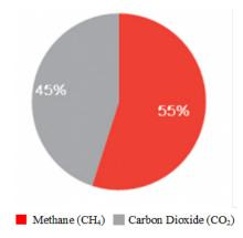
Fig. 1. Biogas composition from agricultural residue
