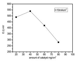
**Figure 4.** Optimization curve of the catalytic mass amount at a constant ratio for the ORR (catalyst: PTFE) = 80:20.
