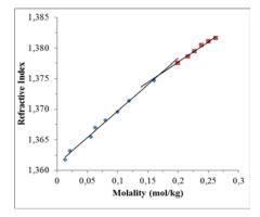
**Figure 6.** Refractive index *versus* concentration plot for SV in ethanol at 288K.
