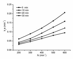
Figure 5. Effect of the rotational speed of the impeller on the volumetric mass transfer coefficient for orifice submergence depth of 0.25 m and gas-free liquid level of 0.35 m.
