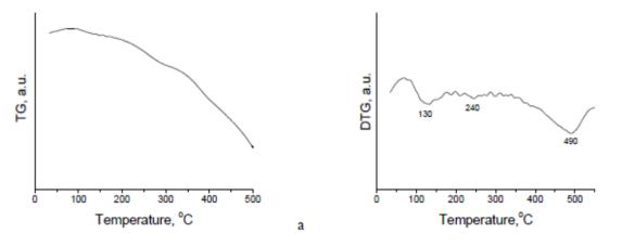
Fig. 2. TPR-TG (a) and TPR-DTG (b) profiles of manganese-modified activated carbon.
