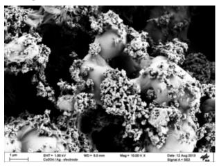
Figure 2. SEM picture of an Ag /Co<sub>3</sub>O<sub>4</sub> mixture.
