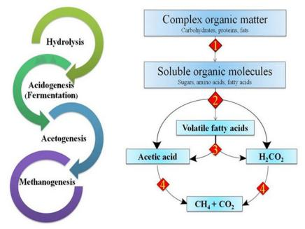
Fig. 2. Process of anaerobic digestion
