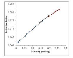
**Figure 5.** Refractive index *versus* concentration plot for LP in ethanol at 288K.
