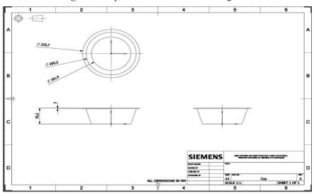
Fig. 6. The top, side and front view of cups
