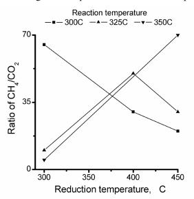
Fig. 1. Selectivity ratio dependence on reduction and reaction temperature for  $(10\%Co+0.5\%Pd)/TiO_2(ox)$  sample.
