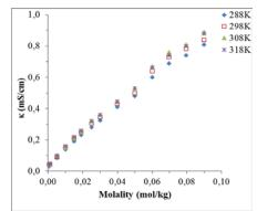
**Figure 3.** Electrical conductivity *versus* concentration plots for SV in ethanol at different temperatures.
