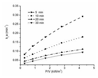
**Figure 7.** Effect of power consumption per unit volume of the liquid on the volumetric mass transfer coefficient for orifice submergence depth of 0.20 m and gas-free liquid level of 0.30 m.
