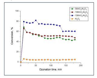
**Fig. 2.** Ozone conversion as a function of ozonation time for varying manganese oxide contents in the catalyst samples.
