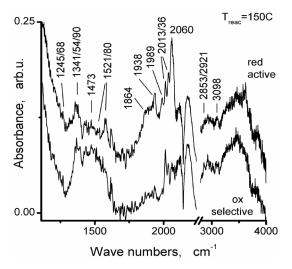
Fig. 6. In situ DRIFTS during CO hydrogenation.
