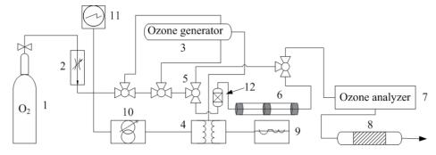
Fig. 1. Experimental set-up for catalytic decomposition of ozone: 1 - oxygen; 2 - flow controller; 3 - ozone generator; 4
