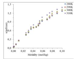
**Figure 1.** Electrical conductivity *versus* concentration plots for CPAM in ethanol at different temperatures.
