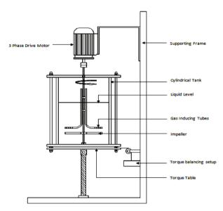
Figure 1. Experimental setup of the gas inducing mechanically agitated contactor.
