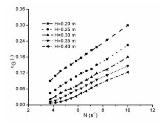
**Figure 3.** Effect of the rotational speed of the impeller on fractional gas holdup in water for an air-inducing tube set with 6 tubes along with a six-bladed straight-blade turbine impeller for bottom clearance of 0.10 m for a straight-blade turbine impeller and 0.10 m for an airinducing tube set.
