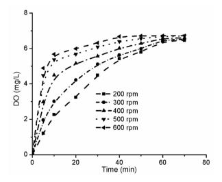
**Figure 4.** Effect of the rotational speed of the impeller on the dissolved oxygen concentration of water for orifice submergence depth of 0.20 m and gas-free liquid level of 0.30 m for different impeller speeds.
