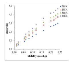
**Figure 2.** Electrical conductivity *versus* concentration plots for LP in ethanol at different temperatures.
