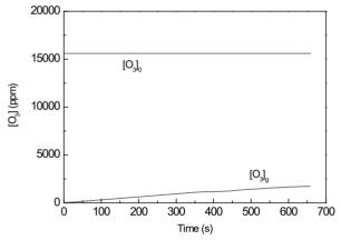
Fig. 1. Dependence of the ozone gas phase concentration ( $[O_3]$ ) in the ozone-oxygen mixture on bubbling time: 1% solution of cyclohexanol in CCl<sub>4</sub>, gas feeding rate  $-1.3 \times 10^{-3}$  l.s<sup>-1</sup>, temperature  $-24^{\circ}$ C,  $[O_3]_{\circ}$  – ozone concentration in the reactor inlet,  $[O_3]_{g}$  - ozone concentration in the reactor outlet.
