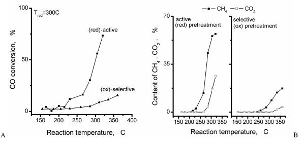
**Fig. 5.** Catalytic behaviour in CO hydrogenation of differently pretreated (10%Co+0.5%Pd)/TiO<sub>2</sub> catalysts: A - CO conversion, B - products distribution.
