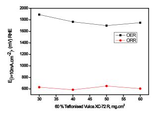
Figure 3. Optimization curve for a quantity of 60 % Teflonized Vulcan XC-72 in mg cm<sup>-2</sup> at E ( $_{i = 10 \text{ mA cm}-2}$ ), mV versus RHE.
