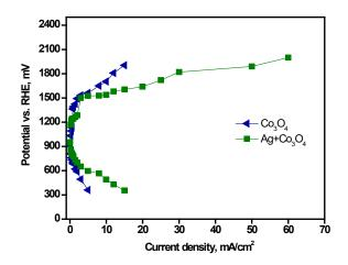
**Figure 6.** Polarization curves of the electrodes for ORR and OER for catalysts:  $\blacksquare$  Ag + Co<sub>3</sub>O<sub>4</sub>;  $\bigvee$  Co<sub>3</sub>O<sub>4</sub>. The electrolyte was 6 M KOH at room temperature. The geometrical area of the electrode was 25 cm<sup>2</sup>.
