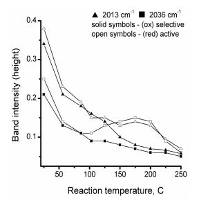
**Fig. 7.** Dependence of some infrared band intensities on reaction temperature.
