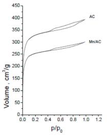
**Fig. 1.** Nitrogen physisorption (-196 °C) isotherms of the activated carbon and manganese catalyst.
