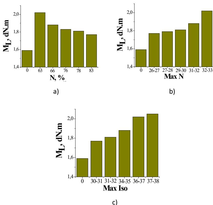
**Fig. 2.** Dependence of the minimum torque of the tested rubber compounds on: a) the amount of normal hydrocarbons in the composition of the wax blends (N); b) the number of atoms in the normal hydrocarbons contained at maximum amounts in the wax blends; c) the number of atoms in the iso-hydrocarbons contained at maximum amounts in the wax blends.
