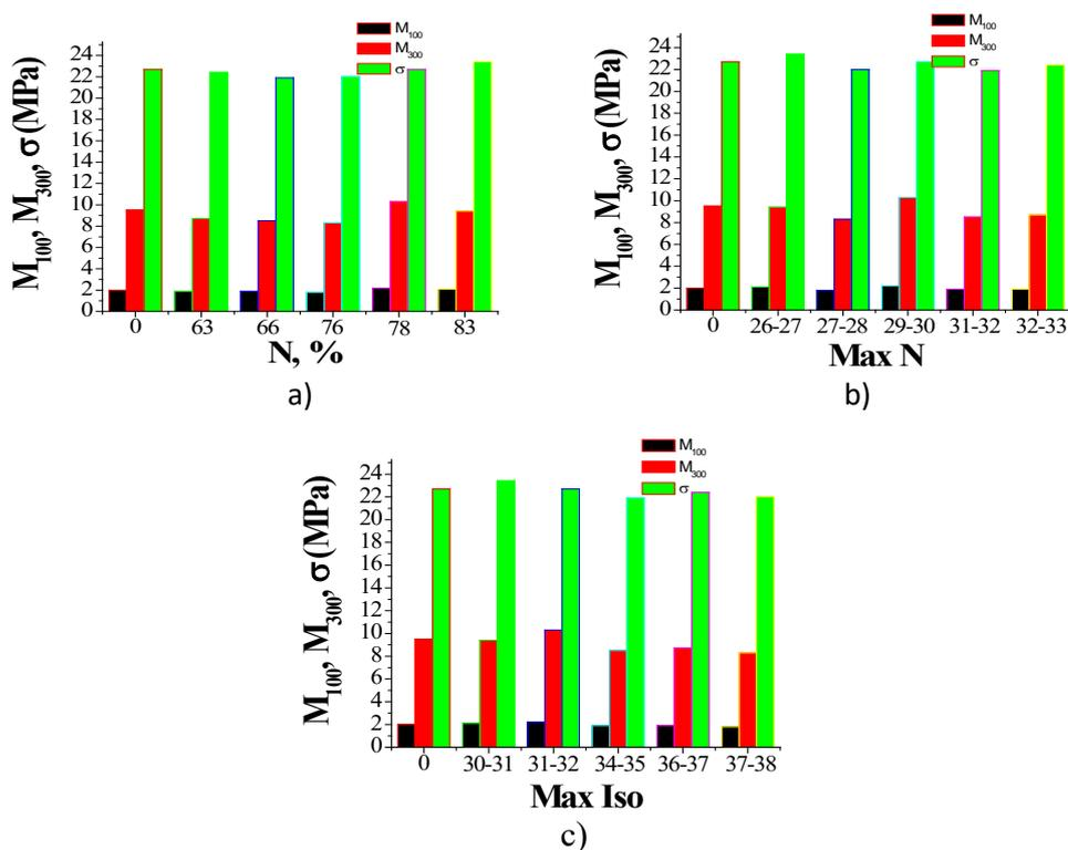
**Fig. 4.** Dependence of physicochemical parameters ( $M_{100}$ -module at 100% deformation, MPa;  $M_{300}$ -module at 300% deformation, MPa;  $\sigma$ -tensile strength, MPa) of the studied vulcanizates on: a) the amount of normal hydrocarbons in the composition of the wax blends (N); b) the number of atoms in the normal hydrocarbons contained at maximum amounts in the wax blends; c) the number of atoms in the iso-hydrocarbons contained at maximum amounts in the wax blends.
