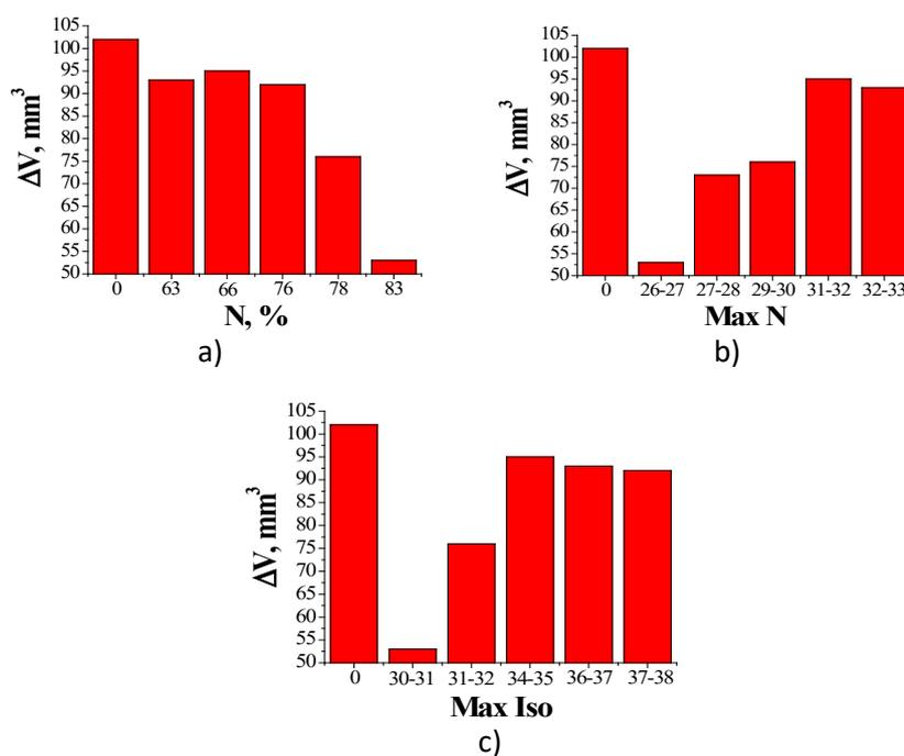
**Fig. 6.** Dependence of the abrasion resistance of the studied composites on: a) the amount of normal hydrocarbons in the composition of the wax blends (N); b) the number of atoms in the normal hydrocarbons contained at maximum amounts in the wax blends; c) the number of atoms in the iso-hydrocarbons contained at maximum amounts in the wax blends.
