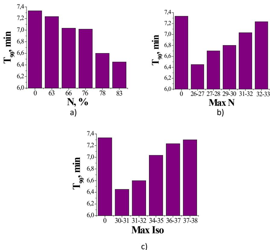
**Fig. 3.** Dependence of the optimal time of vulcanization of the studied rubber mixtures on: a) the amount of normal hydrocarbons in the composition of the wax blends (N); b) the number of atoms in the normal hydrocarbons contained at maximum amounts in the wax blends; c) the number of atoms in the iso-hydrocarbons contained in maximum amounts in the wax blends.
