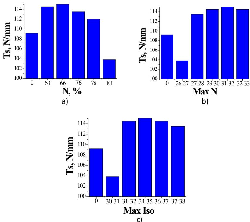
**Fig. 5.** Dependence of the tear resistance of the studied vulcanizates on: a) the amount of normal hydrocarbons in the composition of the wax blends (N); b) the number of atoms in the normal hydrocarbons contained in maximum amounts in the wax blends; c) the number of atoms in the iso-hydrocarbons contained in maximum amounts in the wax blends.
