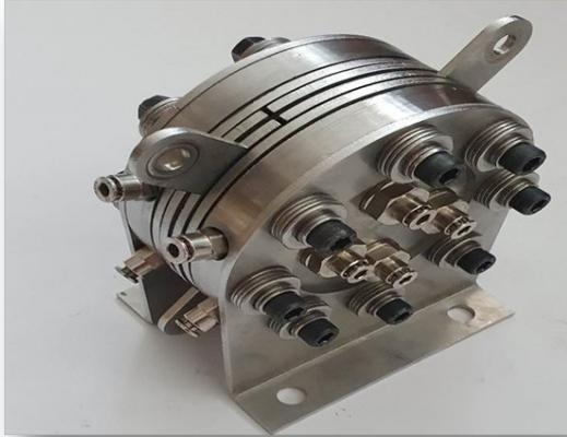
**Fig. 2.** Picture of the self-developed electrochemical hydrogen compressor.
