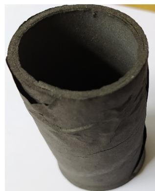
**Fig. 1B.** Pyrolyzed cylindrical carbon tube.
