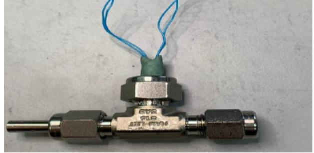
Fig. 2. Assembly of two thermistors in T shape ¼" Swagelok connector
