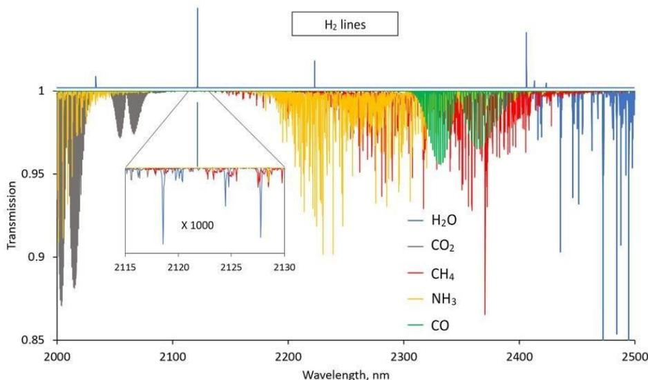
**Figure 10.** HITRAN simulation for the absorption spectrum of various gases and H<sub>2</sub> which might be present in typical usage environments of the sensor [14] open access source.
