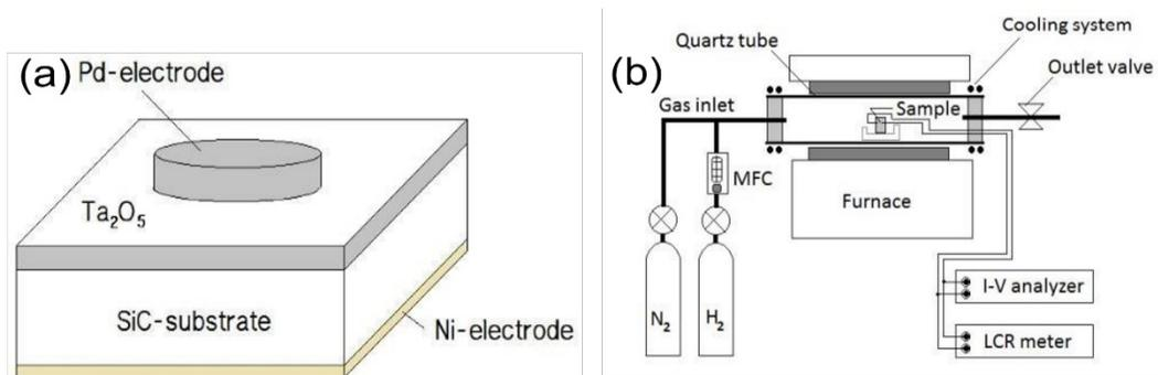
**Figure 5** (a) Pd on SiC substrate with thin layer of Ta<sub>2</sub>O<sub>5</sub>; (b) complete setup for hydrogen sensing [9] open access source.
