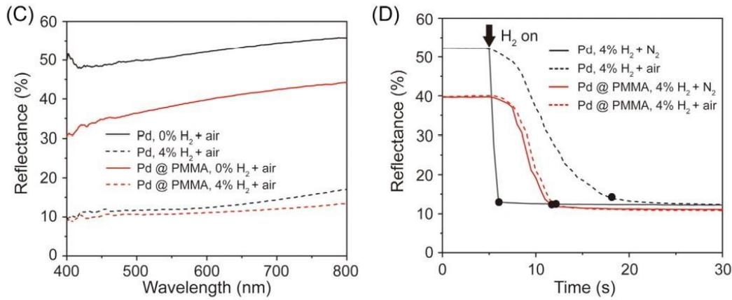
**Figure 8.** (C) Reflectance spectra as function of wavelength of the PPBE and a Pd film on PDMS when exposed to 0% and 4% H<sub>2</sub> mixed with dry air, respectively. (D) Reflectance change as function of time at a fixed wavelength of 600-nm of a PPBE (red line) and a Pd film on PDMS (black line) on exposure to 4% H<sub>2</sub> mixed with N<sub>2</sub> (solid line) and dry air (dash line), respectively [10] open access source.
