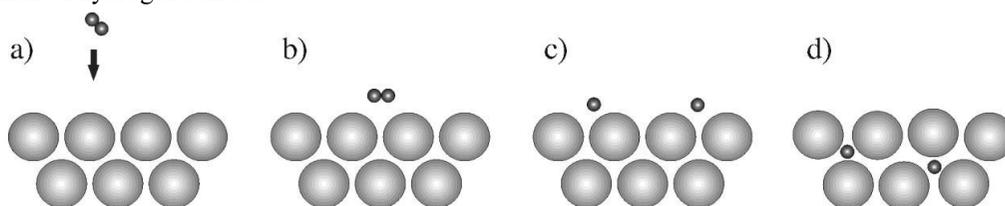
**Figure 2.** Reaction steps between hydrogen molecule and Pd [2].
