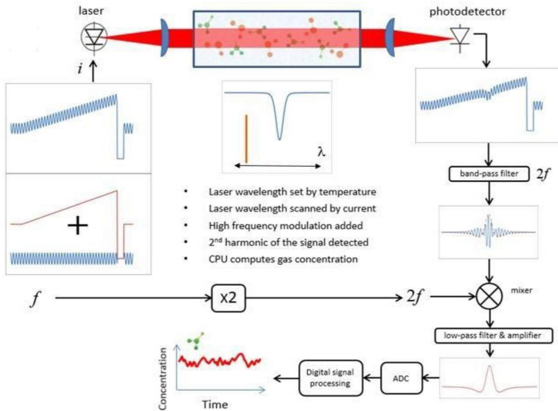
**Figure 9.** Typical arrangement for a spectroscopy-based H<sub>2</sub> gas sensor [14] open access source.
