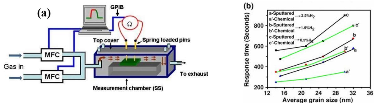
**Figure 4 (a)** Typical H<sub>2</sub> electrical sensing experiment setup; **(b)** Response time of Pd nanoparticles thin films prepared by electrochemical and sputtering technique of thickness 150 nm as function of grain size [4] open access source.
