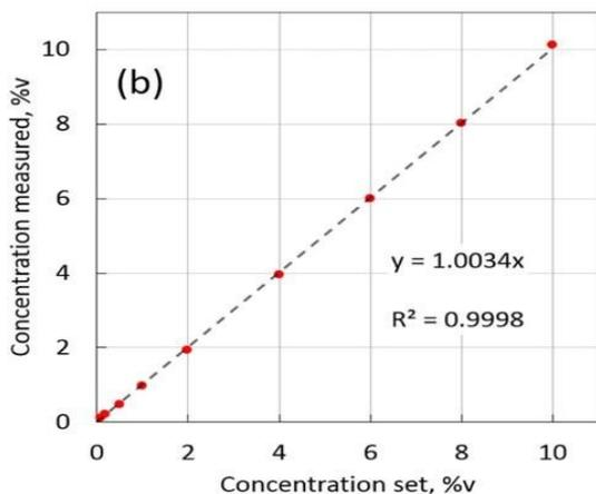
**Figure 11.** Graph of concentration of H<sub>2</sub> in chamber with detection precision [14].
