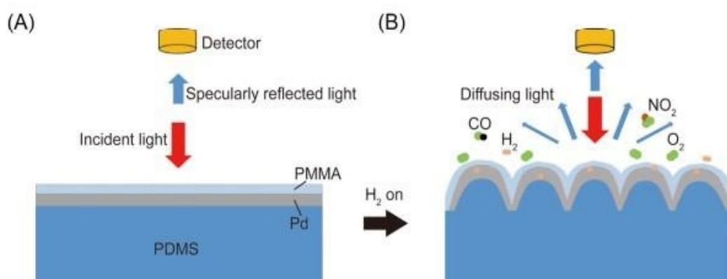
**Figure 7.** Schematic exhibiting the sensing mechanism of the PPBEs. (A) The specularly reflected light by the flat Pd/PMMA bilayer before hydrogenation and (B) diffused reflectance by the wrinkling surface generated by volume expansion of Pd thin film after hydrogenation [10]- open access source.
