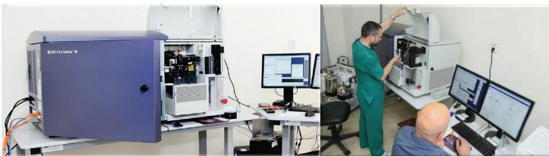
**Figure 3.** Cell Sorter based on 4 laser multiparameter flow cytometry.
