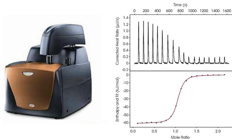
**Figure 12.** Affinity ITC, TA Instruments – detects interaction between protein/DNA/antibody and drug (ligand), works with solutions, cell volume (190  $\mu\text{l}$ ), syringe volume (250  $\mu\text{l}$ ), temperature range (2–80  $^{\circ}\text{C}$ ), measured heat range (0.04–5000  $\mu\text{J}$ ).
