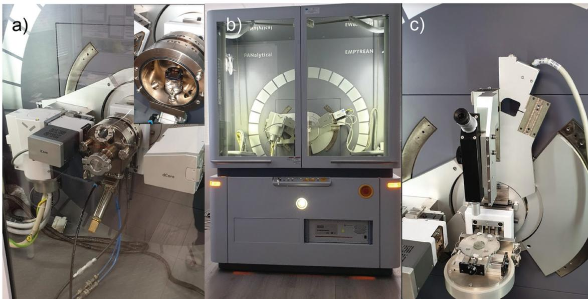
**Figure 10.** Diffractometer Empyrean. Applications: qualitative phase/polymorphs and quantitative analysis (wt%), Cu (1.5406 Å) and Co (1.7902 Å) sources; modes: reflection, transmission, microdiffraction (spot of 50 μm), measurements at different temperatures and different gas environments, low temperature (to -200 °C), high-temperature (to +600 °C), controlled atmosphere, SAXS/USAX, thin layers (up to 500 nm), microdiffraction, xyz stage etc.
