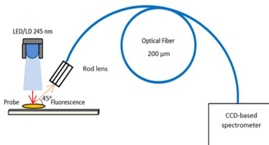
**Fig. 1.** Mobile experimental installation used by fluorescence spectroscopy
