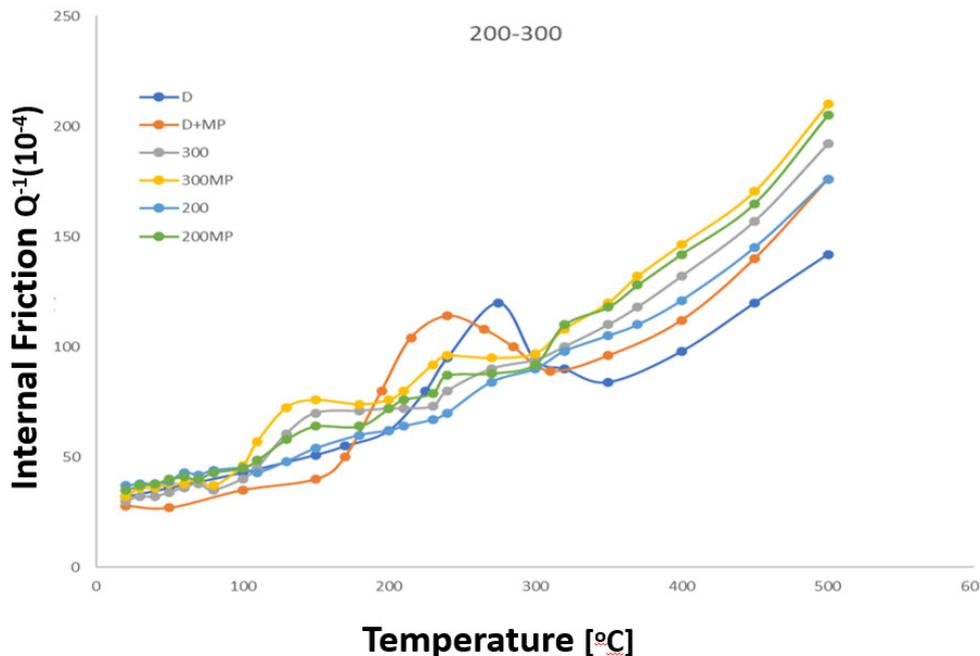
**Fig. 4.** Summary graph of temperature dependences of internal friction after: D - 10% deformation without annealing, after annealing 200°C and 300°C. Lines 200 and 300 without pulsed magnetic field; D+ MP, 200MP, 300MP - in a pulsed magnetic field.
