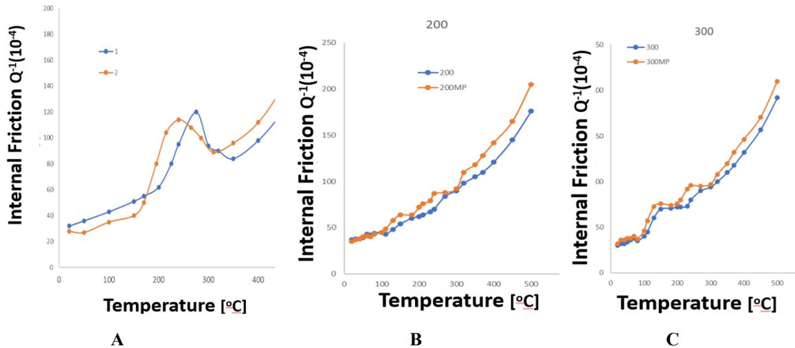
**Fig. 3.** Temperature dependence of internal friction in aluminum (purity 99.99%): A-deformation 10% without annealing; annealing at temperature: B-200°C; C -300°C. Curve 1 - without pulsed magnetic field; curve 2 - in a pulsed magnetic field.
