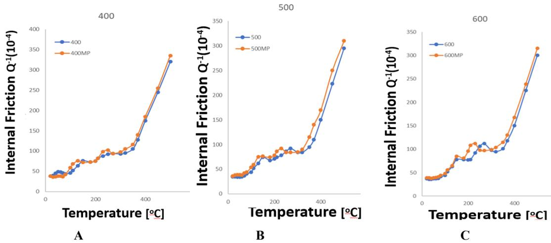
**Fig. 5.** Temperature dependence of internal friction in aluminum (purity 99.99%) after annealing at temperature: A-400°C; B-500°C; C-600°C. Curve 1 - without pulsed magnetic field; curve 2 - in a pulsed magnetic field.
