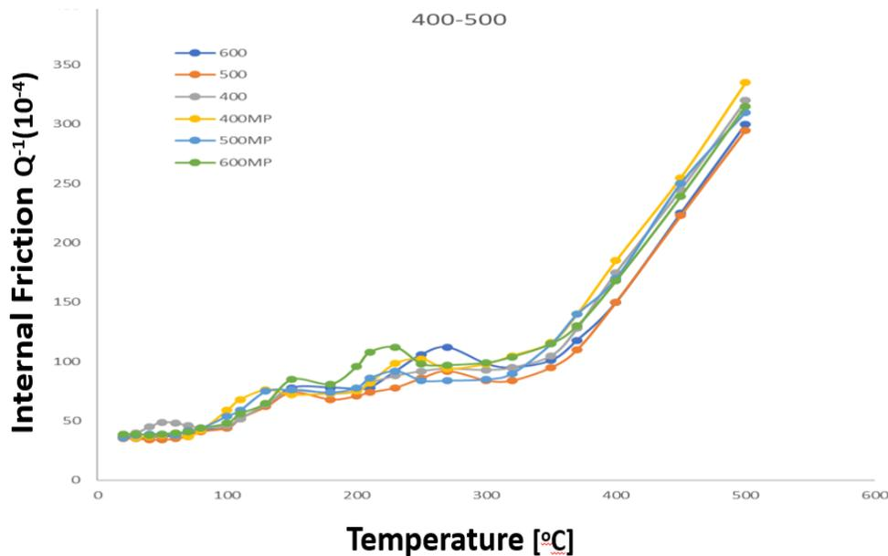
**Fig. 6.** Summary graph of temperature dependences of internal friction after deformation of 10% and annealing at temperatures of 400°C, 500°C, and 600°C. Curves 400, 500, and 600 without pulsed magnetic field; curves 400MP, 500MP, 600MP - in a pulsed magnetic field.
