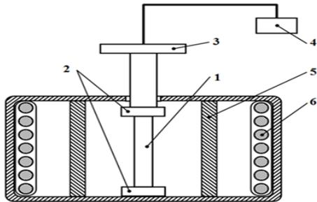
**Fig. 1.** Setup to study the effect of a pulsed magnetic field on a material, simultaneously with heat treatment. 1- sample; 2- clamps; 3- inertial detail; 4- counterweight; 5- heating chamber; 6- magnetic solenoid.
