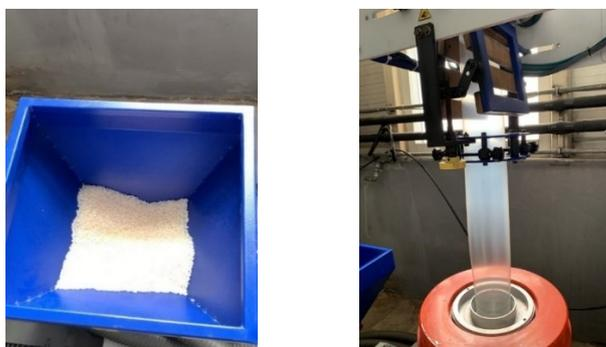
**Fig. 1.** Images of PHAs bioblend granules and blown film production
