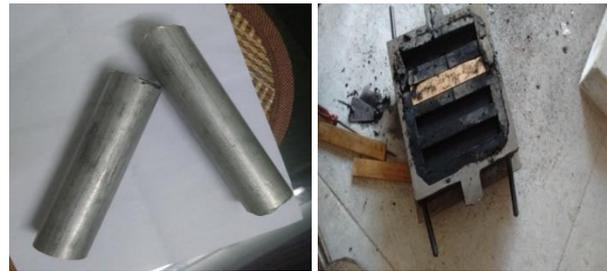
**Figure 1.** Aluminum base material and mold
