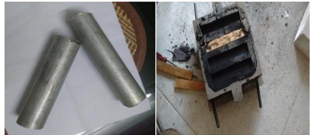
**Figure 1.** Aluminum base material and mold
