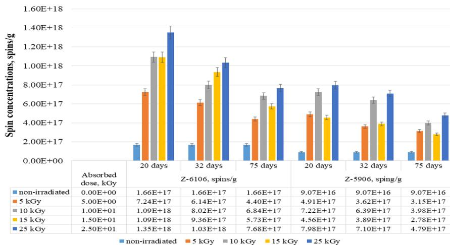
**Fig. 2.** Change of the spin concentrations of the ebony wood samples with time, before and after gamma irradiation with 5, 10, 15 and 25 kGy at standard (1 Gy/s) dose rate.
