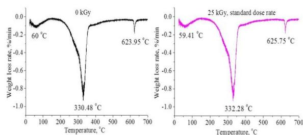
**Fig. 7.** DTG diagrams of ebony sample Z-5906 before and after gamma irradiation with 25 kGy at standard dose rate.
