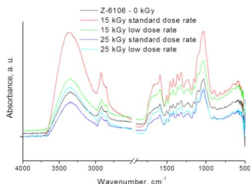
**Fig. 4.** FTIR/ATR spectra of the ebony wood sample Z-6106 before and after gamma irradiation with 15 kGy and 25 kGy at low and standard dose rate.
