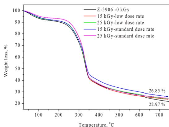
**Fig. 5.** TGA curve of the ebony wood sample Z-5906 before and after gamma irradiation with 15 and 25 kGy at low and standard dose rates.
