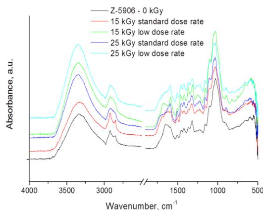
**Fig. 3.** FTIR/ATR spectra of the ebony wood sample Z-5906 before and after gamma irradiation with 15 kGy and 25 kGy at low and standard dose rate.
