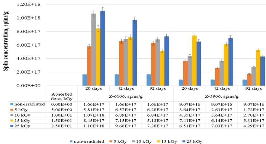
**Fig. 1.** Change of the spin concentrations of the ebony wood samples with time, before and after gamma irradiation with 5, 10, 15 and 25 kGy at low (0.037 Gy/s) dose rate.
