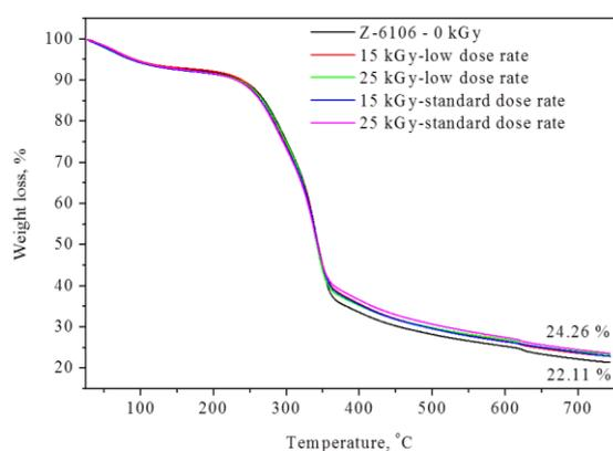
**Fig. 6.** TGA curve of the ebony wood sample Z-6106 before and after gamma irradiation with 15 and 25 kGy at low and standard dose rates.
