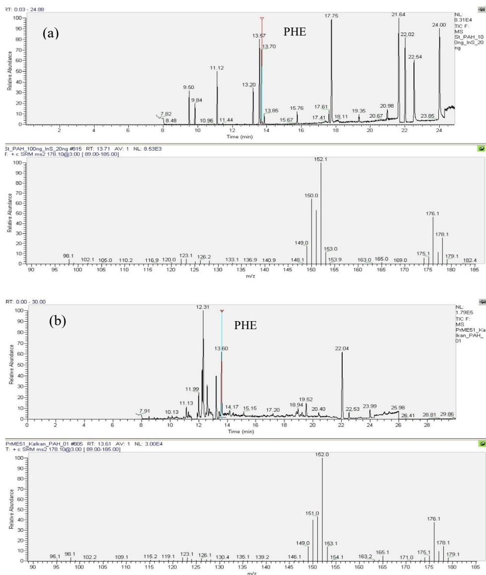
Figure 2. Chromatograms of reference standard solutions of PAHs, 100 ng/mL (a) and fish extract sample (b); mass spectra of PHE in standard and sample.
