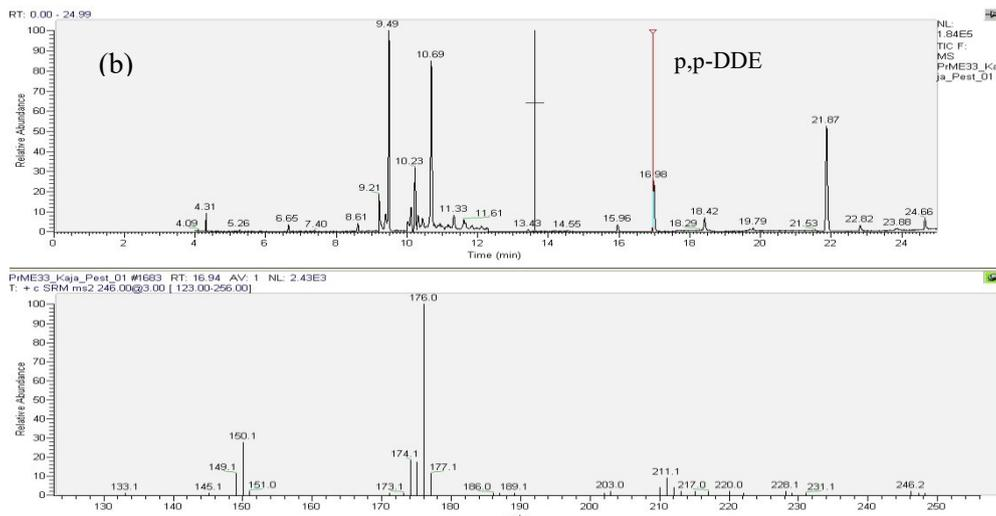
Figure 1. Chromatograms of reference standard solutions of OCPs 100 ng/mL (a) and fish extract sample (b); mass spectra of DDE in standard and sample.
