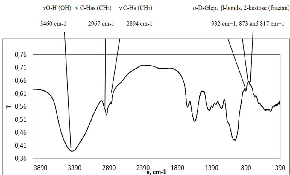
Fig. 4. FT-IR spectrum of shatawari inulin isolated by microwave-assisted extraction with DP 7-10
