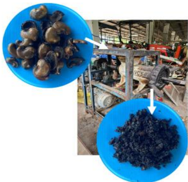
Fig. 2. Using a mincer, grind the cashew nutshells into tiny bits [51]
