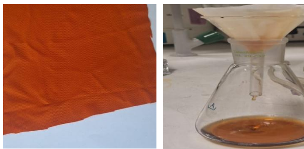
Figure 5 The DO-30 dyed fabric and waste water including DO-30 dye and other dye bath stuffs
