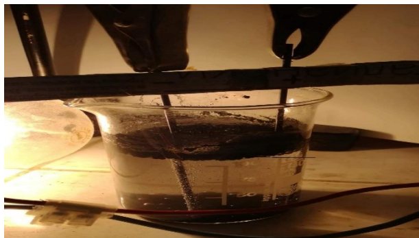
Fig. 4. Photograph of the experimental layout for carrying out the electrolysis
